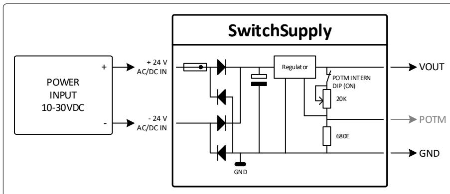
In the example above, a direct current power supply is used and is connected to the Power in connections. The internal potentiometer is used (DIP on **ON**). The external potentiometer is NOT used. The GND of Power in and Power out are isolated from each other.
