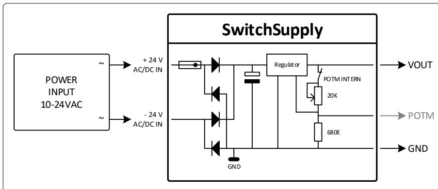
In the example above, an alternating current power supply is connected to the Power in connections. The internal potentiometer is used (DIP on **ON**). The external potentiometer is NOT used.
