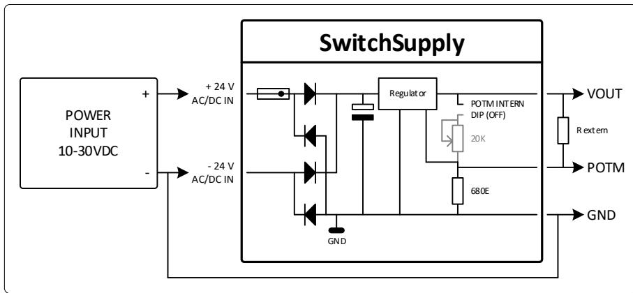
In the example above, a direct current power supply is used and is connected to the Power in connections. To adjust the voltage of Power out an external potentiometer or resistor (R extern) is used. The internal DIP is set to **OFF**, which disables the internal potentiometer.
