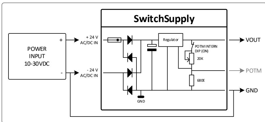
In the example above, a direct current power supply is used and is connected to the Power in connections. The internal potentiometer is used (DIP on **ON**). The external potentiometer is NOT used. The GND of Power in and Power out are linked with each other.
